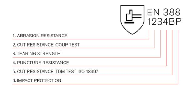
Household waste gloves provide minimum cut protection level 4 and puncture protection level 3. Garden waste gloves provide minimum puncture protection level 3 but preferred level is 4.
